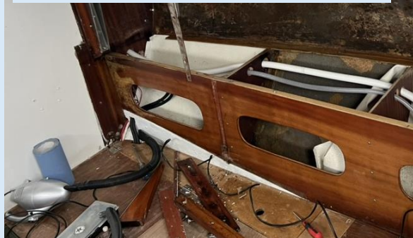
Fitting new stowage with 18 mm bulkhead bolted to original lower bulkhead dividing cubbies, transferring rig loads back to the hull.
