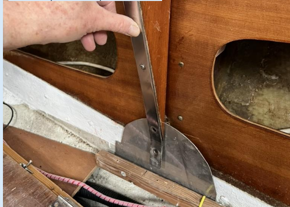
Lower ss strap being refitted with semi-circular plate to spread load.
