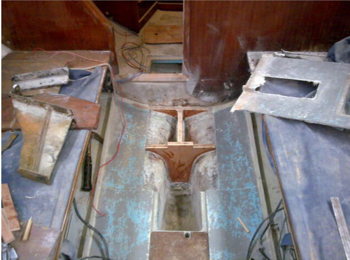
I then used M10 machine screws to tap and glue the Selden mast foot into the oak pad. This was now solid and ready for the mast to be stepped. The whole job cost me 8 hours of my time and £300 for the composite mast step. This is a lot less than the £1500 quoted by a boat yard to do the job.
